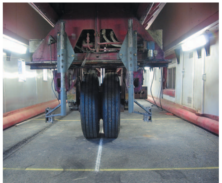
Tensar has carried out years of laboratory research and numerous full scale tests to evaluate the stabilisation effect of Tensar geogrids in flexible pavements.
