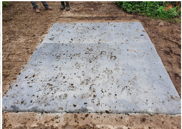
CCX-M TM installation intact after 100 passes
